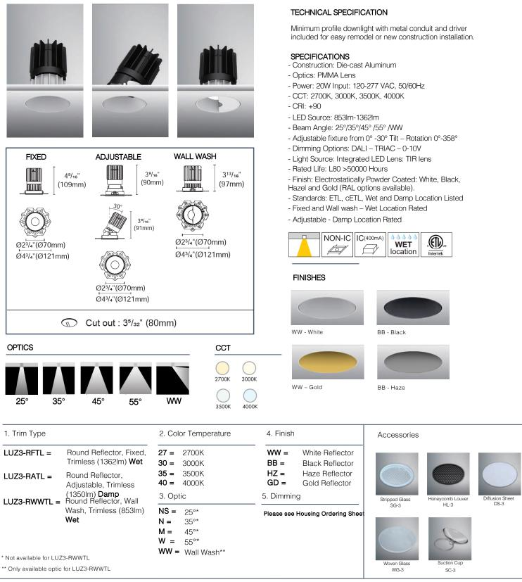
Example: LUZ3-RFTL-30-M-WW = 3" Round Trimless Fixed Downlight – 3000K – 45° Optic – White Reflector
