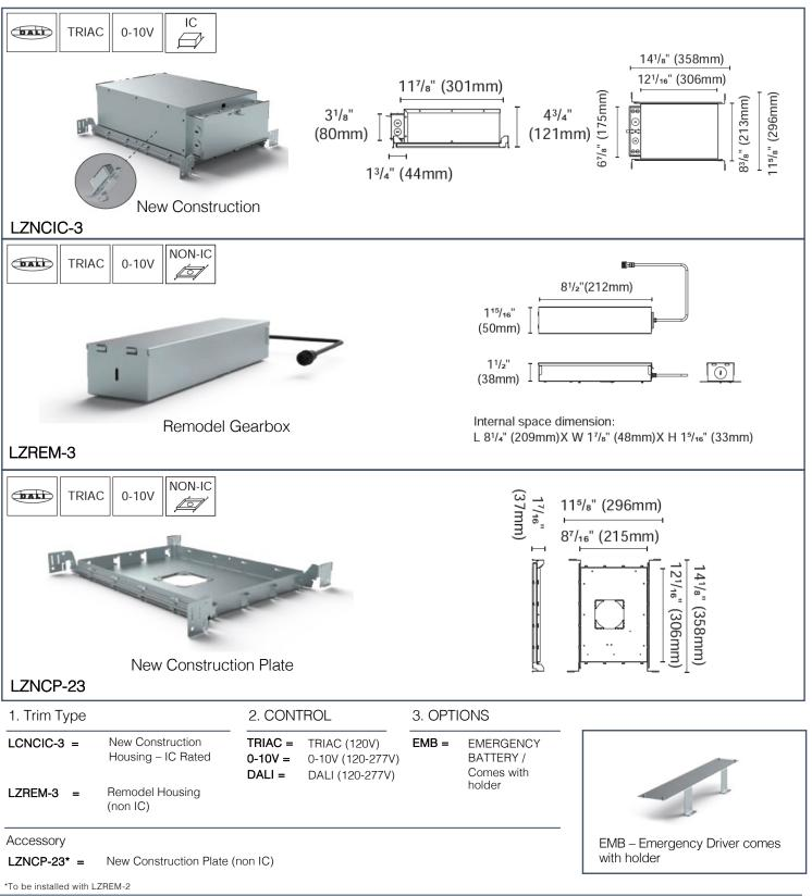
Example: LCNCIC-3-TRIAC = New Construction Housing – Triac Dimming
