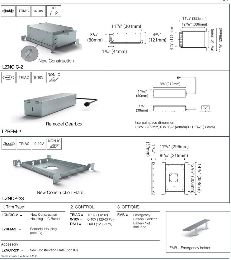
Example: LCNCIC-2-TRIAC = New Construction Housing – Triac Dimming
